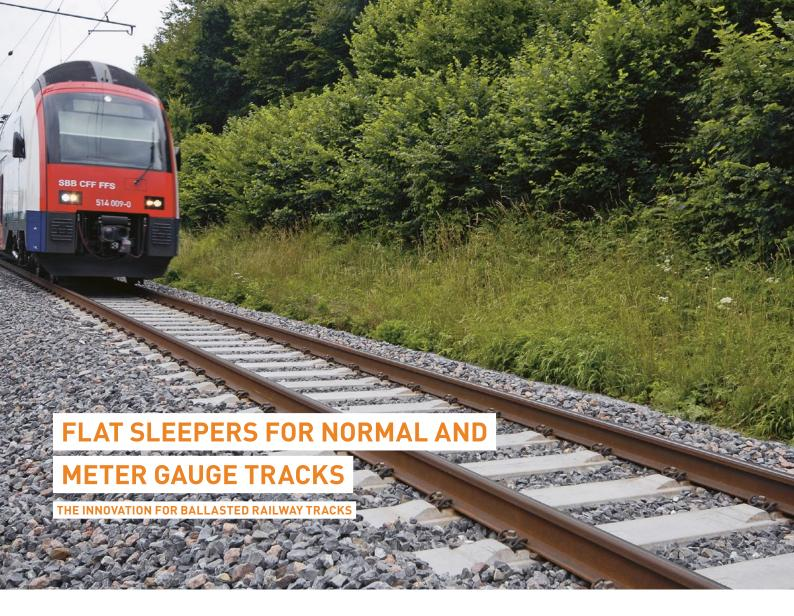
The flat sleeper increases the economic efficiency of ballasted track. It is available for normal and meter gauge railway tracks and offers all the advantages of standard concrete mainline sleepers. At the same time the superstructure requires less maintenance.
